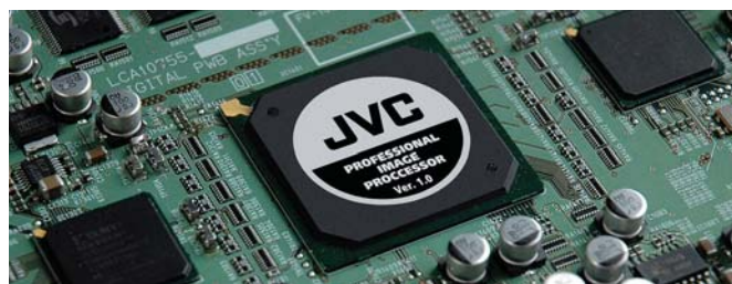
JVC's new 10-bit, real time digital image processor
