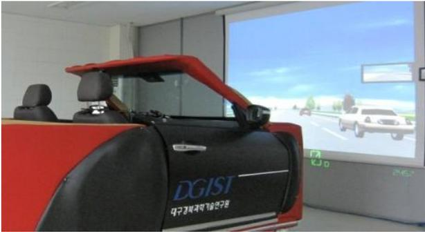
Fig. 1 Fixed-based Driving Simulator
