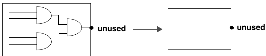
Figure 6-5 Minimizing Logic Driving an Unconnected Output Port
